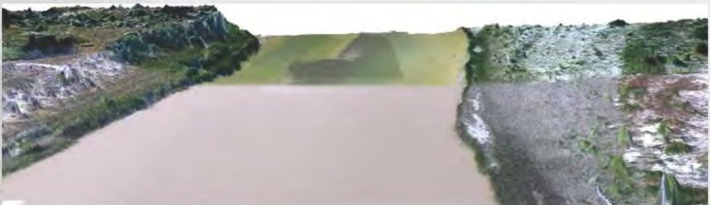
Figure 15. 3D image model developed from close-range photogrammetry along the Powder River, Wyoming. Images from two different times of year are merged to highlight the change in vegetation. With the 3D information available from multi-temporal 3D dataset, changes in vegetation heights, bank erosion, slope, water depth, vegetative cover, and bare ground can be measured (Noble et al. 2008).
